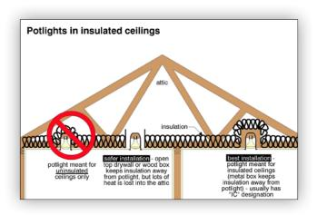
visible to the home inspector. Where pot lights are used in an insulated cavity, an electrician should be engaged to verify the safety of the system.
