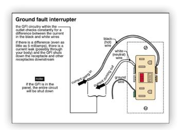
Modern electrical codes require ground fault protection where there is the potential for water to come into contact with electricity. This includes receptacles for bathrooms, kitchen countertops, wet bars, laundry tubs, spas and hot tubs, whirlpool baths, swimming pools, unfinished basements and outdoor receptacles.
