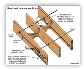
overheated in the past as a result of over-fusing, a poor connection or damaged cable. Often the wire becomes brittle in high heat areas, such as panels and junction boxes. In exposed areas, where inspection is easy, there is usually good air circulation and little heat build-up. The wires are least likely to be brittle in these areas.
