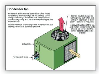
noisy, especially attic fans as the noise is transmitted through the rafters and ceilings. Bad bearings can also make the fan noisy. Fans may be inoperative due to belt or pulley problems, a failed electric motor, or interrupted electrical supply.
