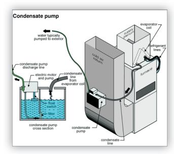
**POOR DISCHARGE** Condensate should not discharge **LOCATION FOR** into plumbing fixtures where CONDENSATE siphoning problems may develop. Condensate should not discharge into the space below a floor slab or into a plumbing stack, in most cases. Condensate should not run down the outside of the building wall because the wall may be damaged.
