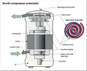
EASILY DAMAGED Severe damage can occur to air conditioning compressors if they are turned on when the outside temperature is below 65° F (16° C). Some compressors contain a small heating element (crankcase heater) that must be on for 12 to 24 hours prior to the compressor starting up. The heater ensures there is no liquid refrigerant mixed in with the lubricating oil. If the heater has not been turned on, or if the outside temperature is low, the compressor cannot be tested.
