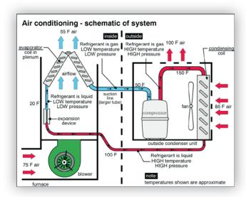
1.1.2 Compressor: The compressor is a pump that moves the refrigerant through the system and compresses the refrigerant when it is a gas, raising its temperature significantly. The compressor is the heart of the system. It is usually located outdoors in the condenser cabinet.
