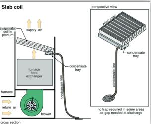
If the water cannot flow by gravity, a condensate pump moves the water to a suitable location. The condensate should not discharge directly into a plumbing vent or stack, or onto a roof.
