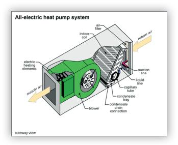
Heat pumps should not be run in the cooling mode when outside temperatures are below 65°F. Above 65°F, heat pumps should not be run in the heating mode.
