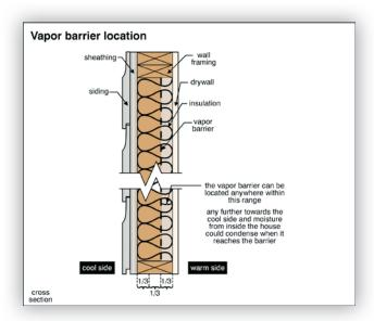
Occasionally, vapor barriers are inadvertently installed on the inside of the wall (vinyl wallpaper, for example), which can lead to water vapor being trapped in the wall and causing mold or rot.
