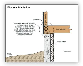
done for another reason, such as damp-proofing the basement/crawlspace walls. This work often includes an egg-crate type drainage layer installed against the foundation wall. Rigid or semi-rigid insulation is added, and the upper portion of the insulation (above ground level) is covered by a protective material such as cement board.
