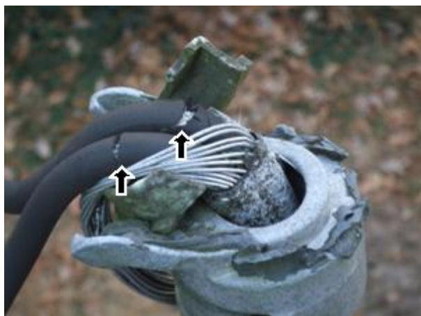
8.0 Picture 3 Split insulation on conductors
